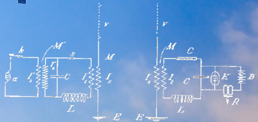
FIGS. 1 AND 2.—DIAGRAM OF CIRCUITS FOR SENDING AND RECEIVING STATIONS.
