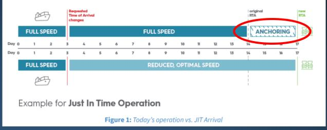
The concept of JIT Arrival of ships allows for ships to optimize their speed during the voyage in order to arrive at the Pilot Boarding Place (PBP) when the availability of Berth, Fairway, Pilot and Nautical services are ensured.
