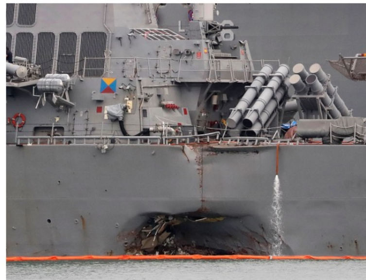
The damaged port aft hull of USS John S. McCain, is seen while docked at Singapore's Changi naval base on Aug. 22, 2017 in ... Show more ▾ WONG MAYE-E, AP
